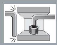
Stubby tools fit in tight spaces where there is not enough overhead clearance for a standard hex key.
