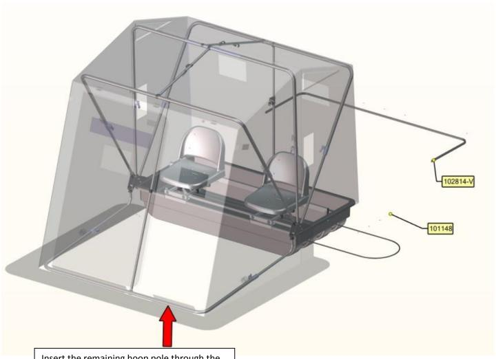
Insert the remaining hoop pole through the sleeve in the front of the tent and attach it to the front 2 poles thus completing the pole assembly.
