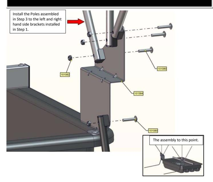
Install the hoop poles, spreader poles, and rope at this time.
