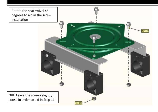
Install the assembly of Step 8 to the seat.
