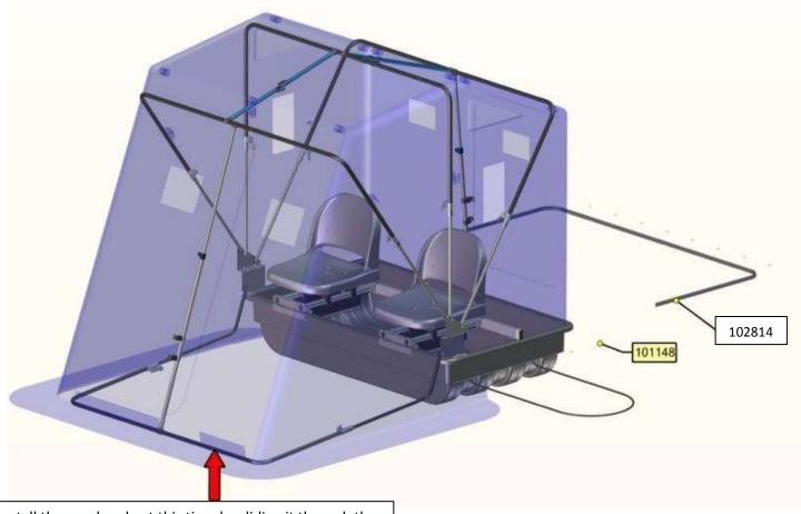
Install the porch pole at this time by sliding it through the sleeve of the tent and then attaching it to the two remaining poles thus completing the pole assembly.
