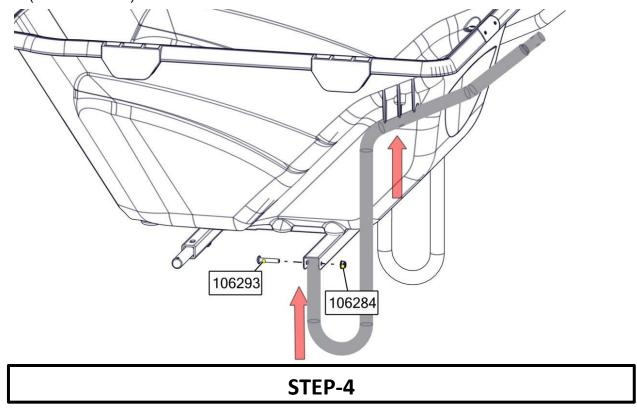
${\bf 1}.\, {\it LOOSELY}$  INSTALL SIDE HANDLE TO BASE AS SHOWN. (BOTH SIDES). IF NEEDED REMOVE FASTENERS FROM PREVIOUS STEP AND RE-INSTALL.
