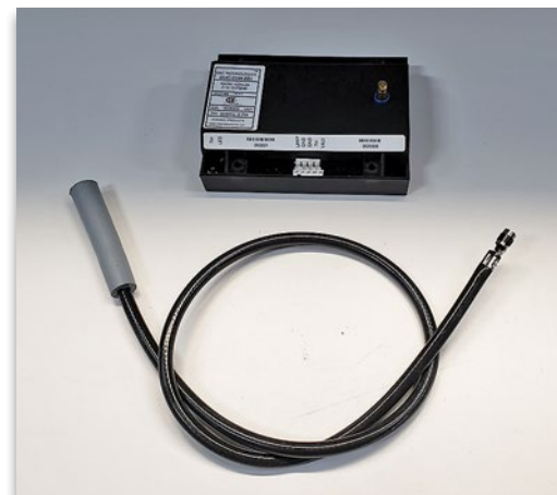
ICM Ignition Control Module or board and high voltage lead
