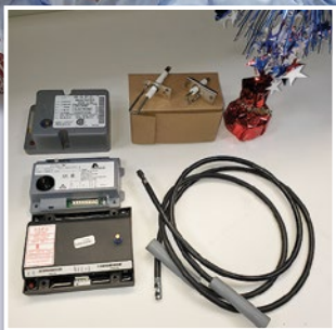
ICMs on left, spark igniters top, high voltage leads right.
