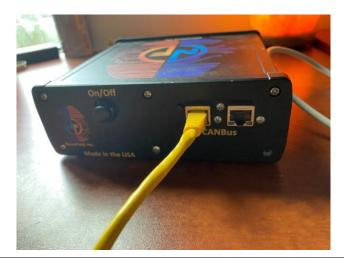
When completed, the Q21 will be connected to the computer. The image below shows the completed connection and, with the EEG Analysis dongle in place is now ready to be used by the NeuroField EEG software.
