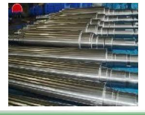
Left are work rolls that will come in contact with the steel.
