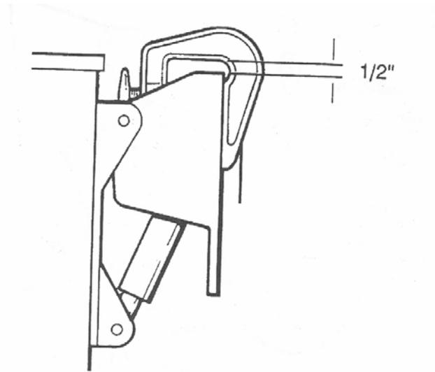
4. Before final installation, slowly run the bracket up to a full tilt to check for interference with the clamp bracket or the clamp handles. Reposition the motor as necessary.
