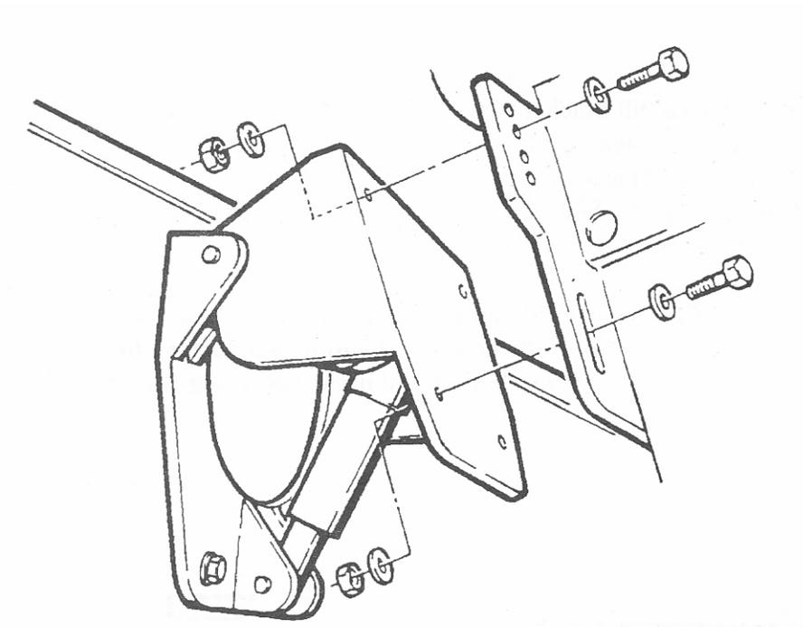
1. The bracket is pre-drilled to fit **most** outboard motor brackets.
