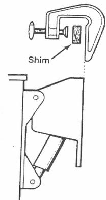
3. Leaving approximately a 1/2 inch space, tighten the clamps securely.
