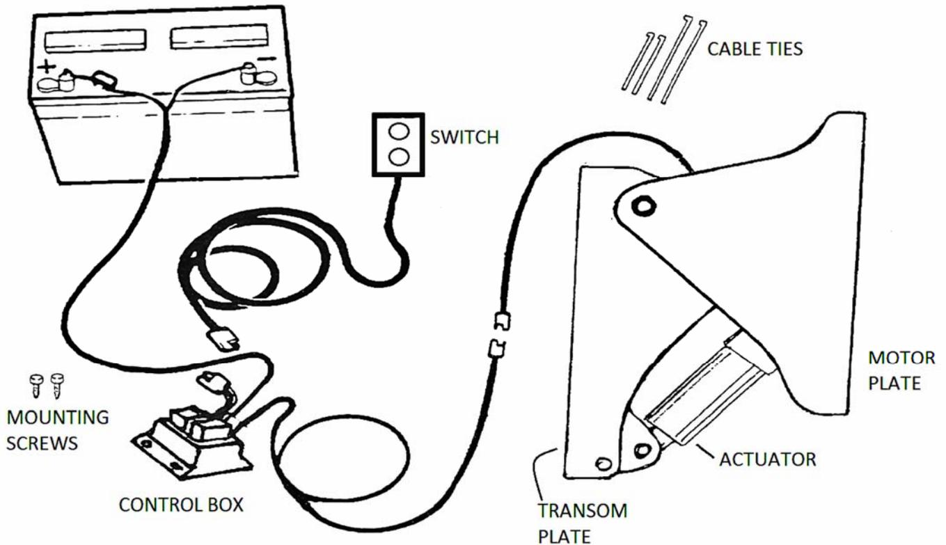
1. Mount the electrical control box inside the boat using the two ½ inch screws provided
