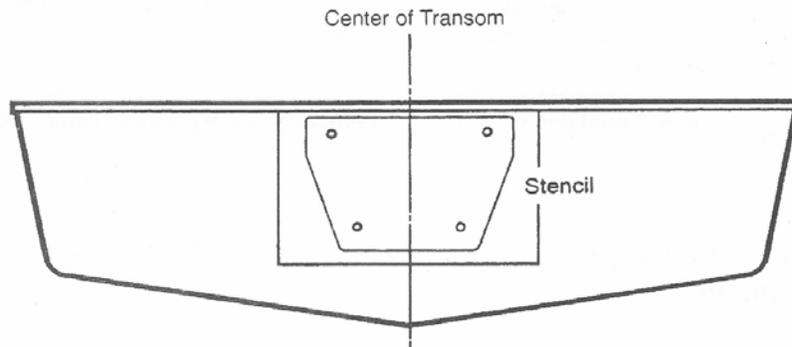
1. Position the transom plate in the center of the transom. Check to make sure that the hole placement will not interfere with any moldings, rivets, etc.
