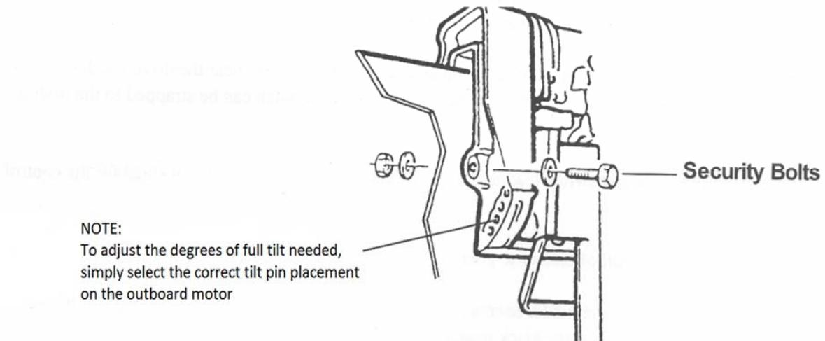
5. Attach security bolts to the bracket by drilling mounting holes into the bracket that match the size and location of the security bolt holes on the outboard bracket. Also use cable ties or other means to secure the clamp handles to prevent accidental loosening during operation.
