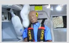
TWO TYPES OF AIRBAGS DEPLOYED
